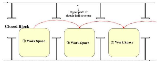
Fig. 6. Closed block structures in double hulled ships
