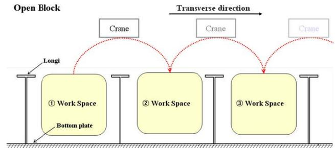
Fig. 5. Open block structure in single hulled ships
