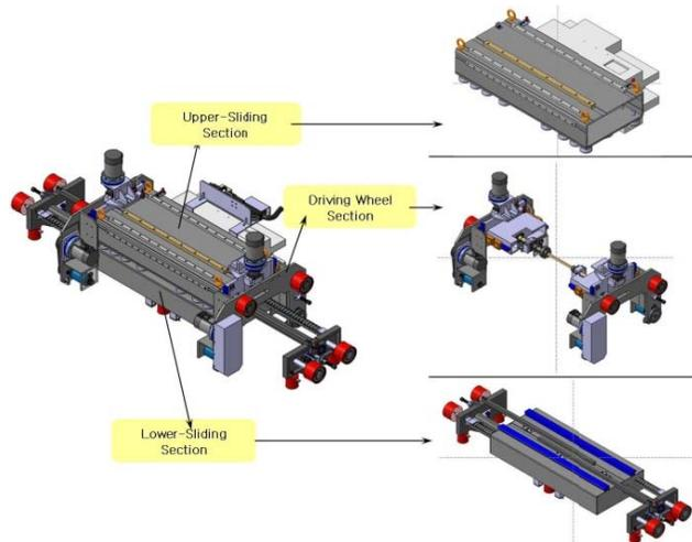
Fig. 8. Arrangement of the overall mechanical set up
