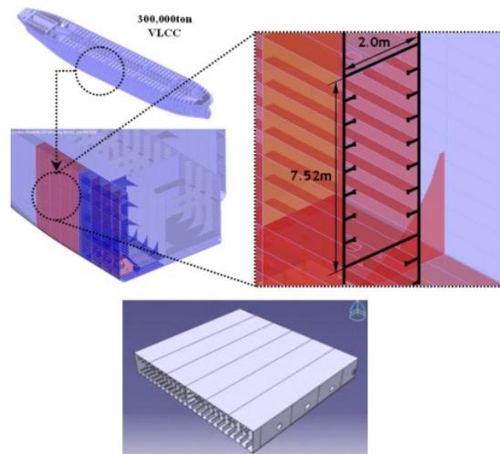
‘Closed Block’ = ‘Double Hull Structure’
