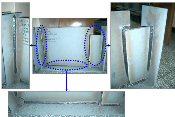
Fig. 19. Welding test results from using the 'Rail Runner'
