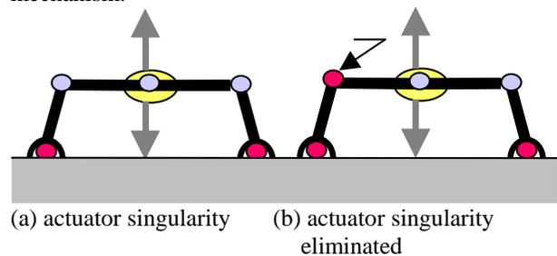
**Figure 8. Adding one more actuator eliminates the actuator singularity.**
