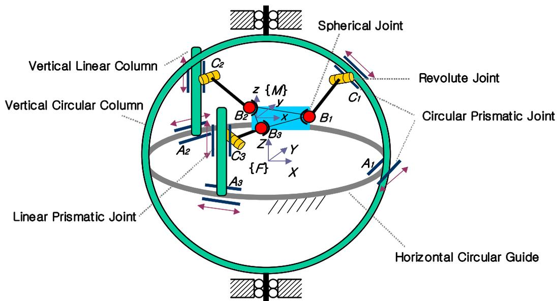
**Figure 3. Architecture of the Eclipse-II mechanism**
