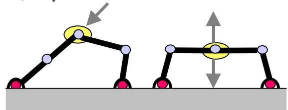
(a) end-effector singularity (b) actuator singularity
