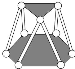
**Figure 1. Structure of Stewart-Gough platform**
