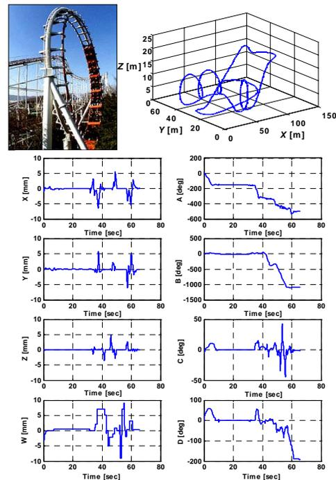
**Figure 11. A scaled model and coordinate values of the roller coaster installed in the Woo-Bang Amusement Park, Daegu, Korea.**
