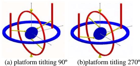
**Figure 5. Examples of the end-effector singular configuration.**
