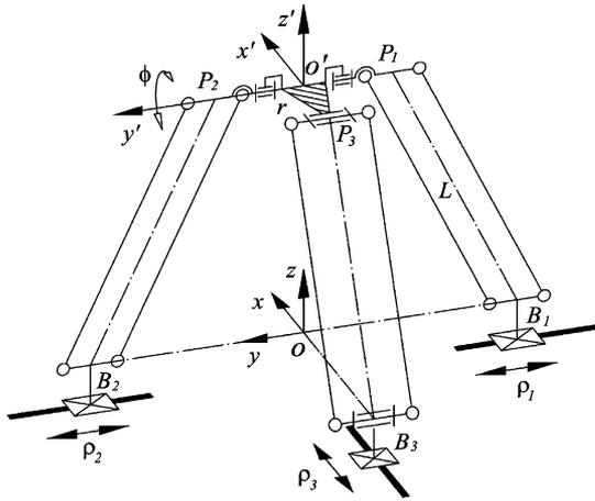
Fig. 2. A kinematics model of the manipulator.
