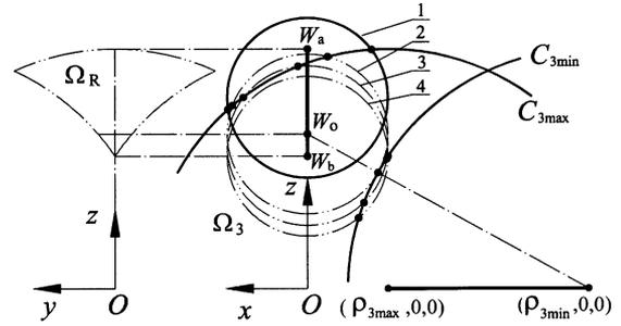
Fig. 7. Intersection classification between circle  $\nu$  and  $C_{3\min}$  and  $C_{3\max}$ .
