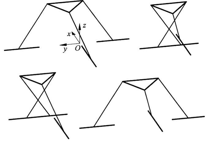
Fig. 8. Four inverse kinematics solutions.
