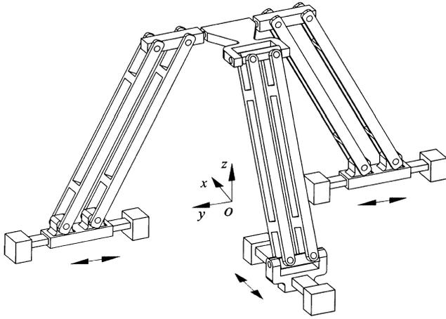
Fig. 1. The new spatial three-DoF parallel manipulator.
