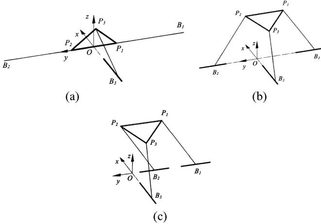
Fig. 5. Three singular configurations of the second kind of singularity. (a)  $P_1B_1$  and  $P_2B_2$  are in the plane  $O-xy$ . (b)  $P_3B_3$  is in the moving platform plane. (c)  $P_1B_1 // P_2B_2$  but neither  $P_1B_1$  nor  $P_2B_2$  is normal to the  $O-xy$  plane and no  $P_3B_3 \perp Ox$ .
