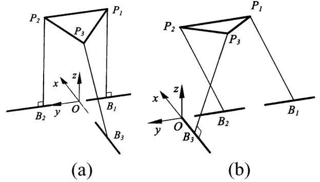
Fig. 6. Two singular configurations of the third kind of singularity. (a) Both  $P_1B_1$  and  $P_2B_2$  are normal to the  $O-xy$  plane. (b)  $P_1B_1 // P_2B_2$  and  $P_3B_3 \perp Ox$ .
