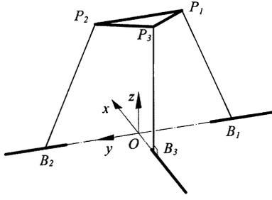
Fig. 4. One example of the first kind of singularity:  $P_3B_3 \perp Ox$ .
