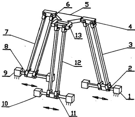
Fig.1 The New Spatial 3-DOF Parallel Manipulator
