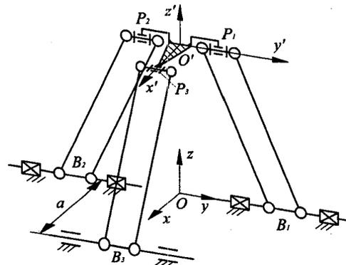
Fig.2 The Geometric Description of the 3-DOF Parallel Manipulator
