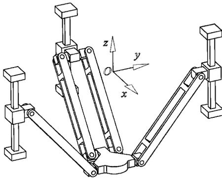
Fig. 1. The *HALF* parallel manipulator presented in ref. [12].
