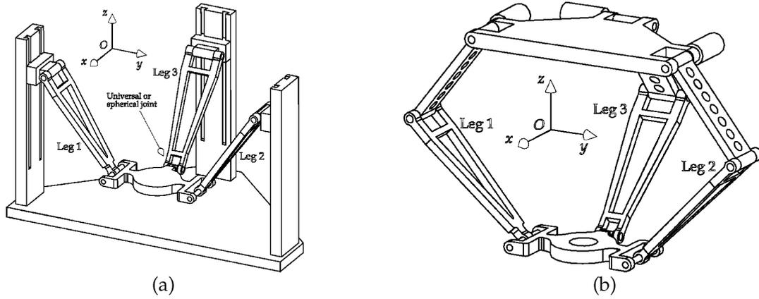
Fig. 6. *HANA\** parallel manipulators: (a) with linear actuators and (b) with revolute actuators.
