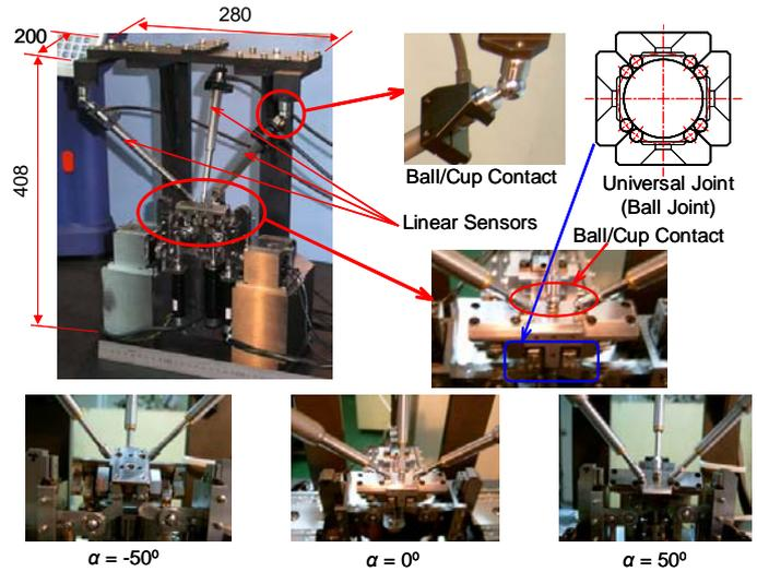
Fig. 2 Micro parallel positioning platform: Sensing part, universal joint and photos of rotation posture
