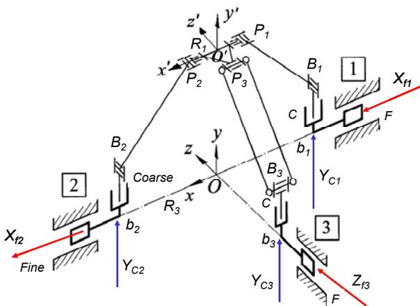
Fig. 1 3-DOF Parallel mechanism and actuation part
