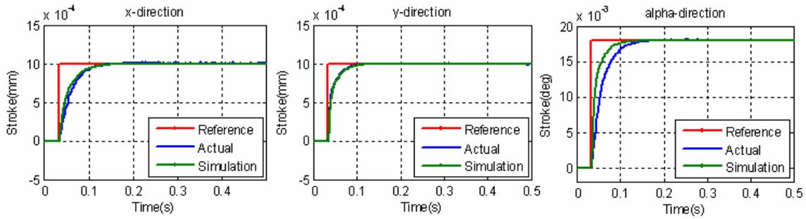
Fig. 7 Verification result of controller by simulation and experiment
