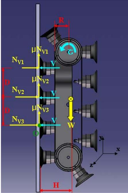
Fig. 4. Forces applied to the robot.
