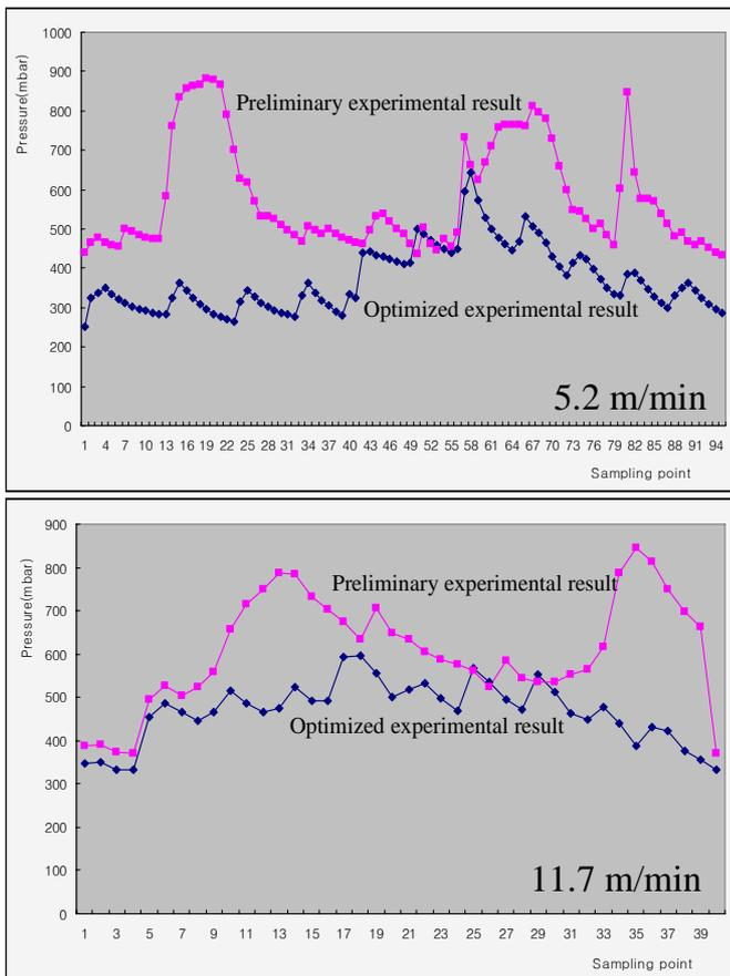
Fig. 11. The optimized results of vacuum pressure.
