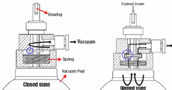
Fig. 2. Working principle of mechanical valve.
