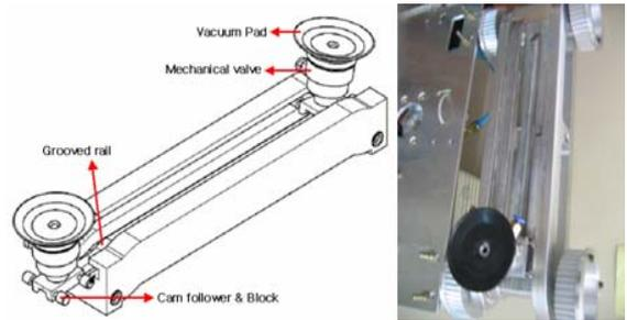
Fig. 3. Feature of cam profile.
