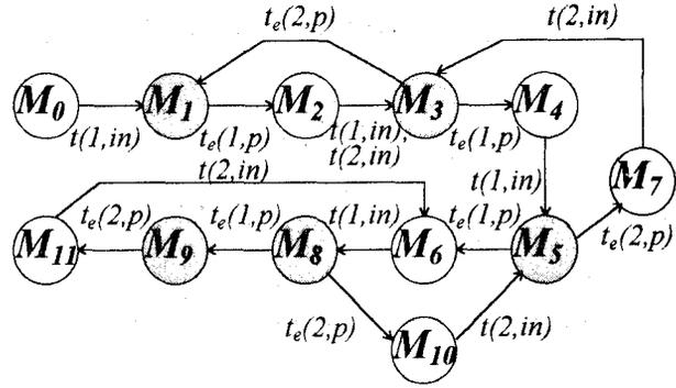
Fig. 5. Reachability graph of the reduced GSPN model of a 2M1B transfer machine with  $n = 4$ .
