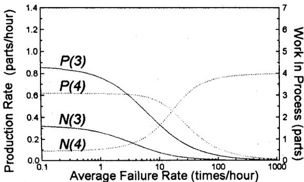
Fig. 8. Effects of the failure rate on the production rate and work-in-process
