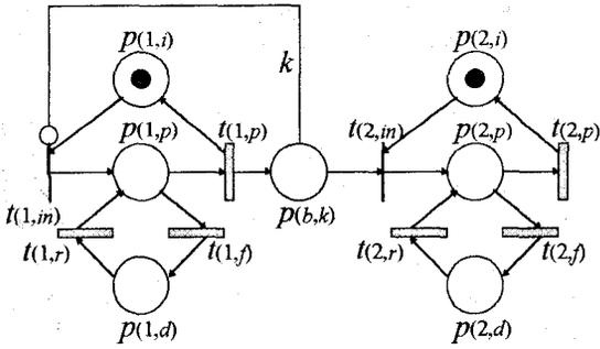
Fig. 3. GSPN model of a 2M1B transfer machine
