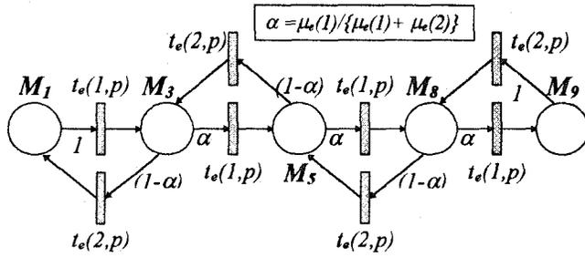
Fig. 6. State machine Petri net in case of the 2M1B transfer machine ( $n = 4$ )
