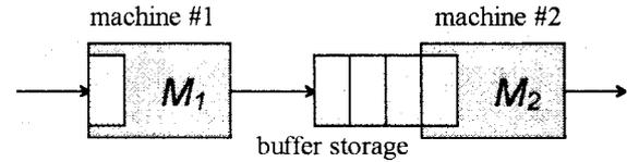
Fig.2. A two-machine one-buffer (2M1B) transfer line
