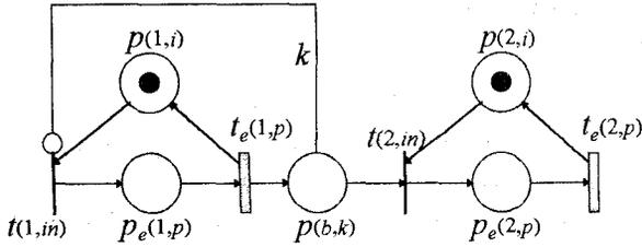
Fig. 4. Reduced GSPN model of a 2M1B transfer machine
