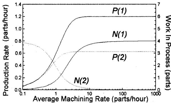
Fig. 7. Effects of the machining rate on the production rate and work-in-process
