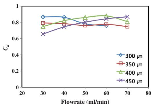
Fig. 6.  $C_d$  of each orifice diameter in single-phase flow.
