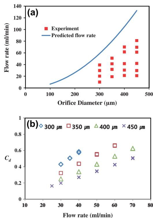
Fig. 7. (a) Comparison of predicted and measured flow rate, and (b)  $C_d$  of each orifice diameter in two-phase flow.
