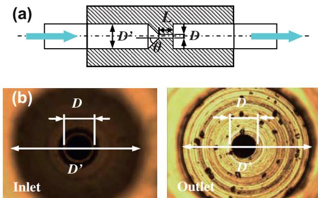
Fig. 5. Orifice design: (a) section view; (b) microscope image of the orifice (350 μm diameter).
