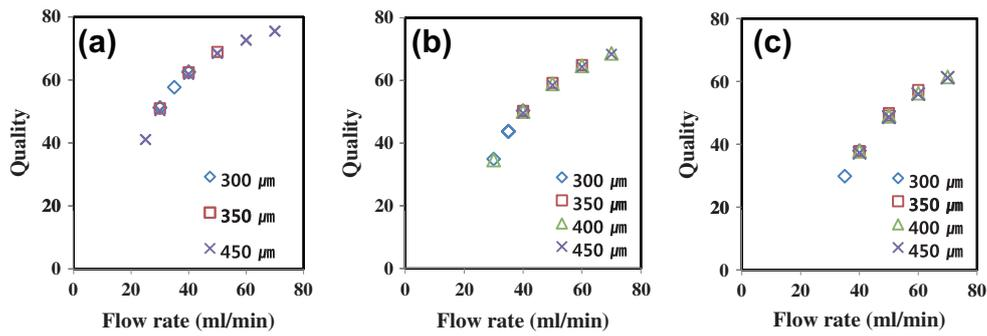
Fig. 8. Relationship between quality and flow rate for each orifice diameter: (a) 60 W, (b) 80 W, (c) 100 W.
