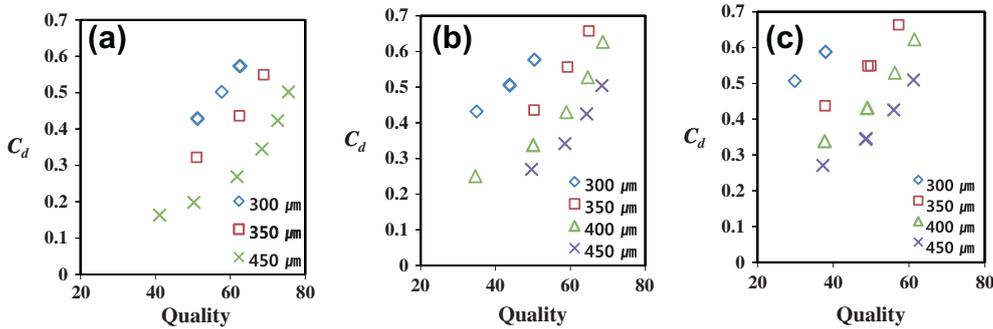
Fig. 9.  $C_d$  for orifices with different cooling loads: (a) 60 W, (b) 80 W, (c) 100 W.
