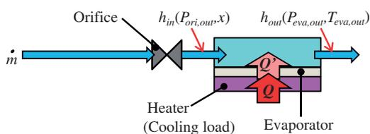
Fig. 2. Diagram of system modeling:  $h_{in}$  and  $h_{out}$  are the enthalpy of the refrigerant at the inlet and outlet of the evaporator, respectively;  $P_{ori,out}$  and  $x$  are the pressure and vapor quality of the downstream flow through the orifice;  $P_{eva,out}$  and  $T_{eva,out}$  are the pressure and temperature at the evaporator outlet;  $Q$  is the cooling load;  $Q'$  is the heat transfer inside evaporator; and  $\dot{m}$  is the mass flow rate.
