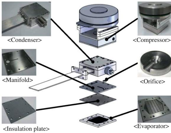
Fig. 1. Design of a small cooling system.
