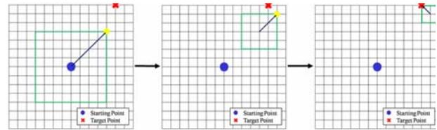
Fig. 5. Example of the branch stretching type exhaustive search method.
