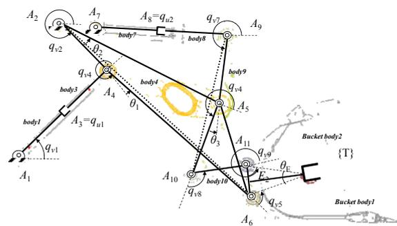
Fig. 3. Front linkage structure and assigned variables.
