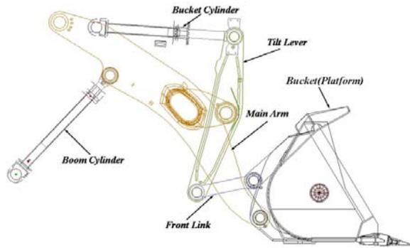
Fig. 1. Nomenclature of the Z-bar wheel loader.
