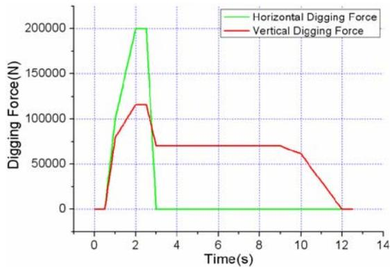
Fig. 6. Force exerted on the bucket.
