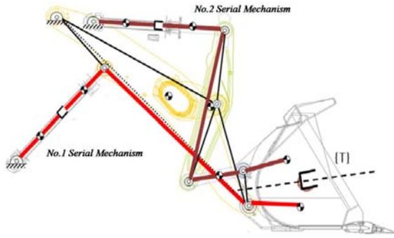
Fig. 4. Schematics of the reduced system of front linkage.
