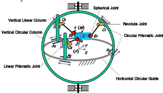
Figure 1. Architecture of the Eclipse-II mechanism
