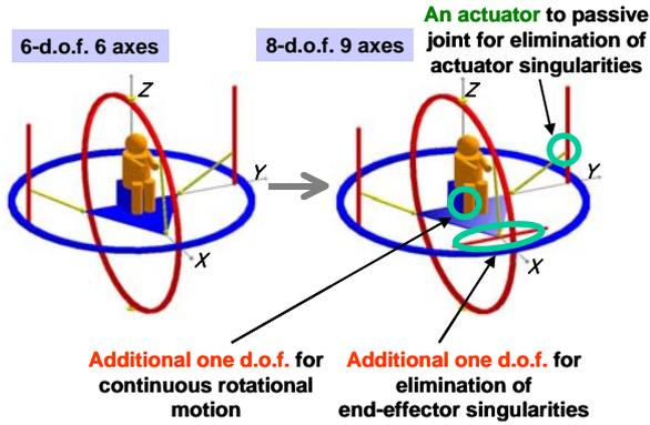
**Figure 6. 8-d.o.f, 9axes Eclipse-II mechanism**
