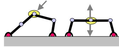
(a) end-effector singularity (b) actuator singularity
