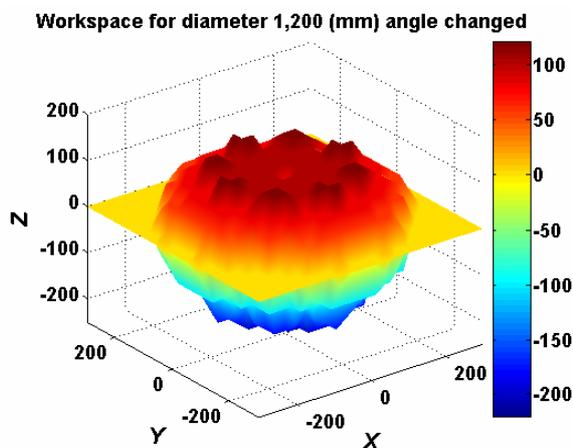
Fig. 11 Workspace of modified Eclipse-II one-man ride machine
