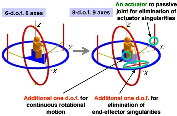
Fig. 6 8-d.o.f, 9axes Eclipse-II mechanism
