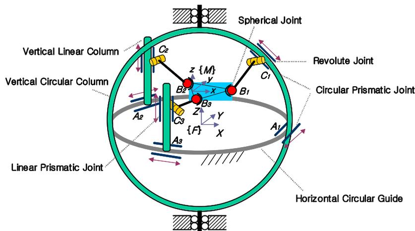
Fig. 1 Architecture of the Eclipse-II 6-d.o.f parallel mechanism
