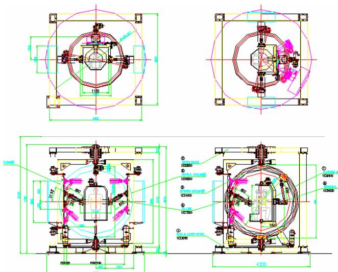
Fig. 8 Assembly drawing of Eclipse-II one-man ride machine
