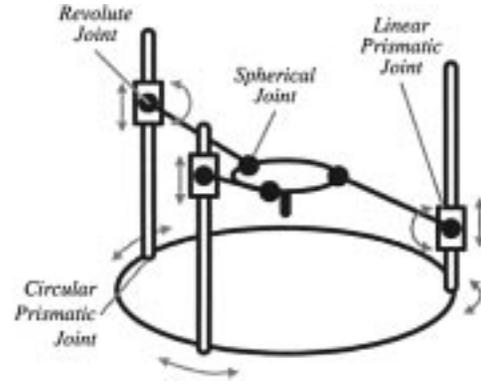
Fig. 3. Final design of the Eclipse.
