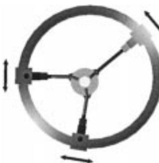
Fig. 5. An end-effector singularity of the Eclipse.
