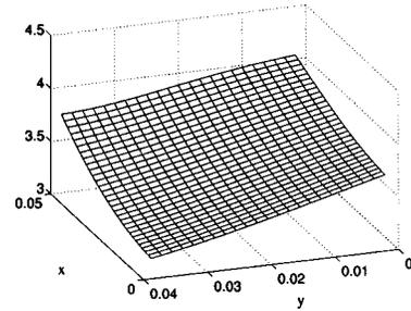
Fig. 13. Frobenius norm of the joint and structural compliance submatrices corresponding to Cartesian position-force stiffness.
