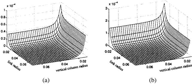
Fig. 15. The compliance measure as a function of the link radius and the vertical column radius. (a) At tilting angle  $0^\circ$ . (b) At tilting angle  $90^\circ$ .
