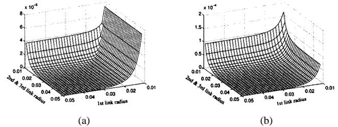
Fig. 14. The compliance measure as a function of the link radius. (a) At tilting angle  $0^\circ$ . (b) At tilting angle  $90^\circ$ .
