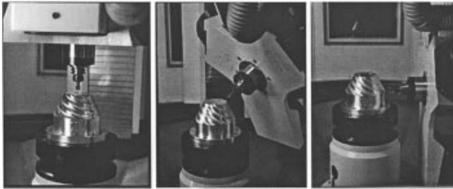
Fig. 18. The Eclipse machine shown machining aluminum stock.
