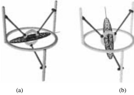
Fig. 12. Compliance ellipsoids for tilting angle  $90^\circ$ . (a) Structural compliance ellipsoid. (b) Joint compliance ellipsoid.
