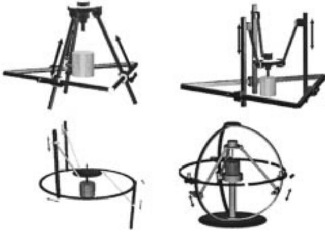
Fig. 2. Conceptual design evolution of the Eclipse.
