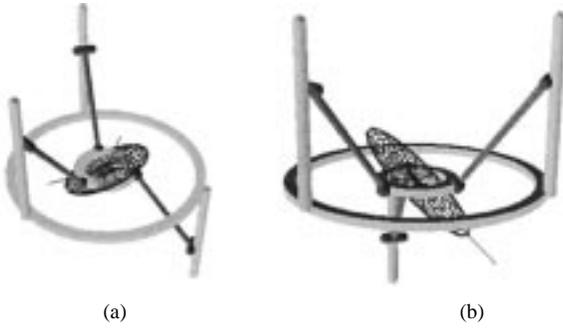
Fig. 11. Compliance ellipsoids for tilting angle  $0^\circ$ . (a) Structural compliance ellipsoid. (b) Joint compliance ellipsoid.
