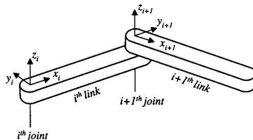
Fig. 10. Serial chain compliance: definition of link frames.
