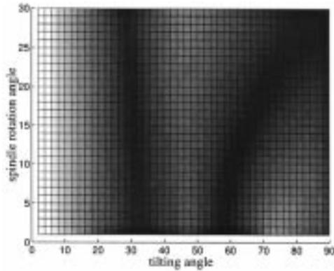
Fig. 6. Singularity barriers of the Eclipse.
