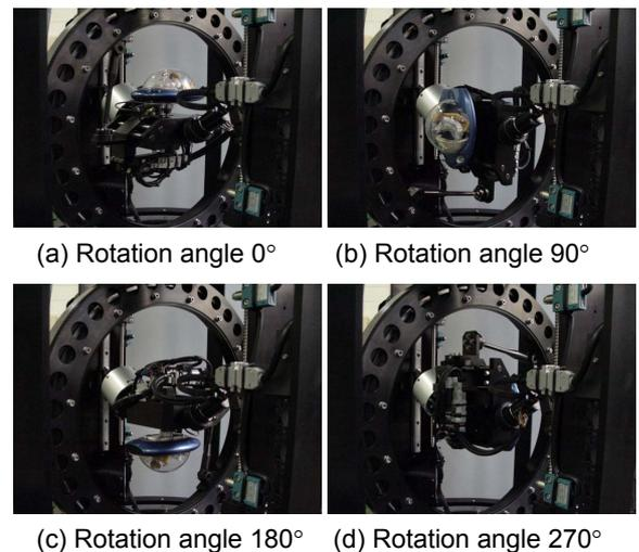
Figure 9: Platform of the Eclipse-II working sample and its 360-degree continuous rotational motion.
