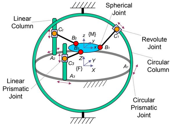
Figure 2: Architecture of the Eclipse-II mechanism.
