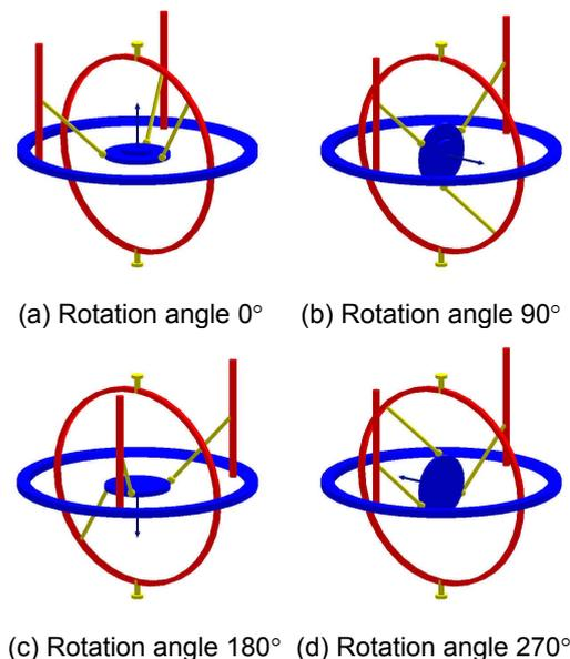
Figure 1: Eclipse-II mechanism and its 360-degree continuous rotational motion.
