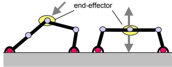
(a) end-effector singularity (b) actuator singularity
