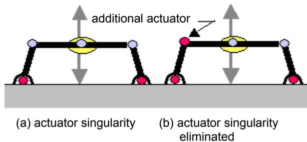
Figure 7: Adding one more actuator eliminates the actuator singularity.
