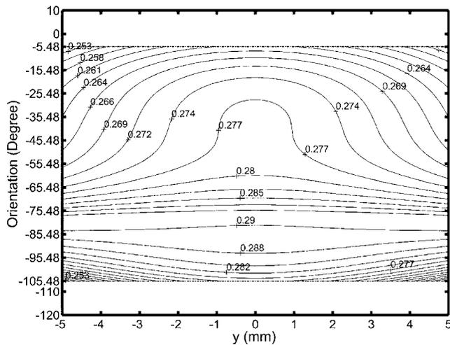
Fig. 10 Distribution of LCI at every section of the desired workspace of the dimensional parallel manipulator
