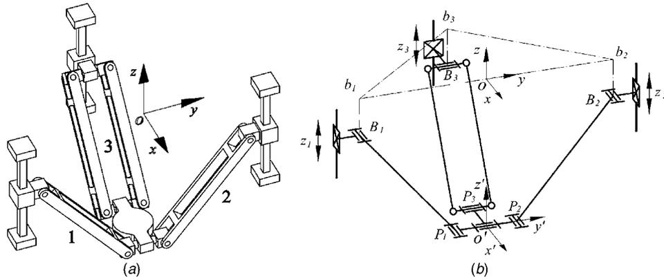
Fig. 1 New spatial 3-DOF parallel manipulator and its kinematical scheme
