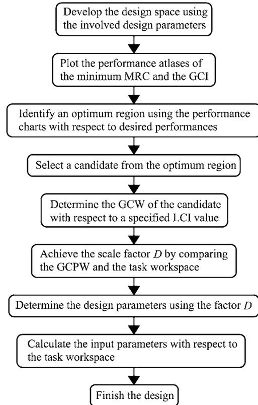
Fig. 11 The flow chart of determination of the link lengths for the 3-DOF parallel manipulator
