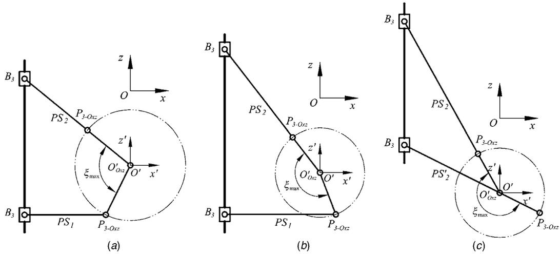
Fig. 2 Three cases of the MRC: (a)  $R'_2 \leq R_3$ ; (b)  $R_3 + R_1 \geq R'_2 > R_3$ ; (c)  $R_3 + R_1 < R'_2$
