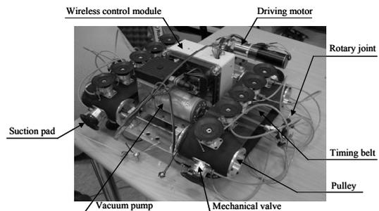
Fig. 1. Overall structure of climbing robot.
