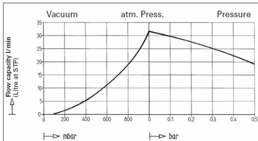
Fig. 7. Performance curve of the vacuum pump..
