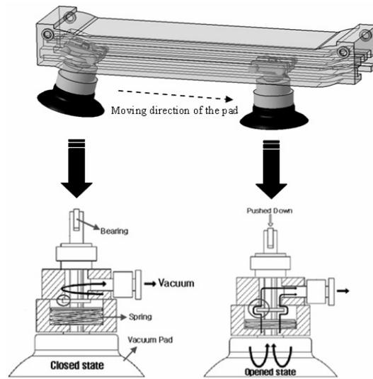
Fig. 4. Working principle of mechanical valve.
