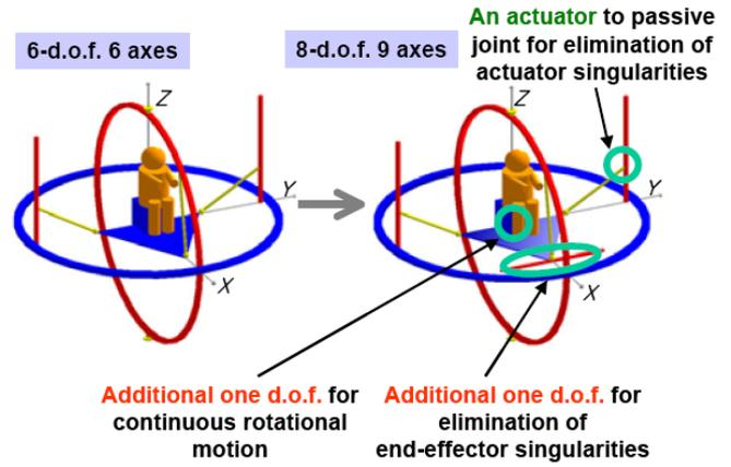
Fig. 2 8-DOF, 9-axis Eclipse-II mechanism
