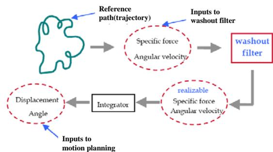
Fig. 6 Procedure of converting the path by the washout filter
