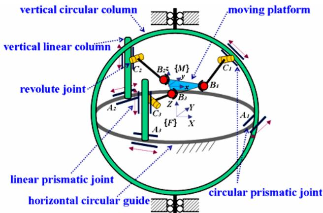
Fig. 1 Architecture of the Eclipse-II mechanism
