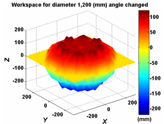
Fig. 10 Workspace of the modified Eclipse-II one-man ride machine
