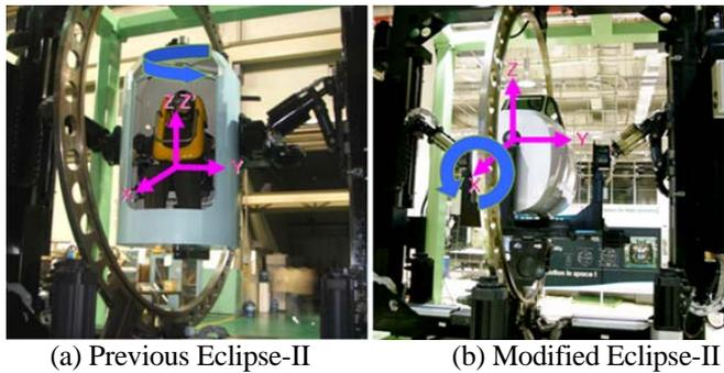
Fig. 8 Rotation axis of the redundant actuator on the chair of the moving platform
