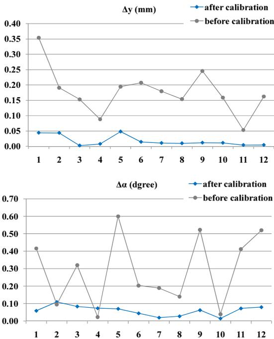
Fig. 5 The result graph of calibration
