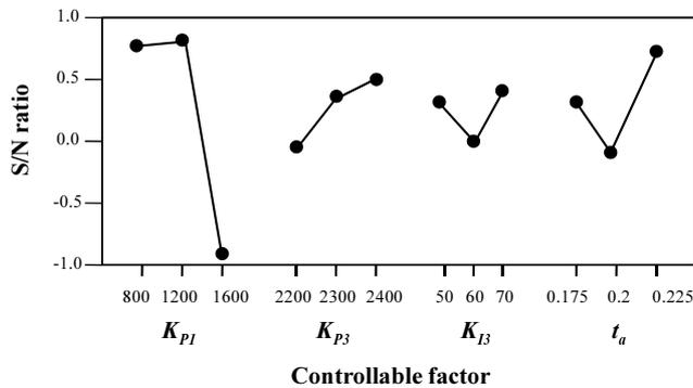
Fig. 11 Response graph obtained at the second optimization experiment for four controllable factors
