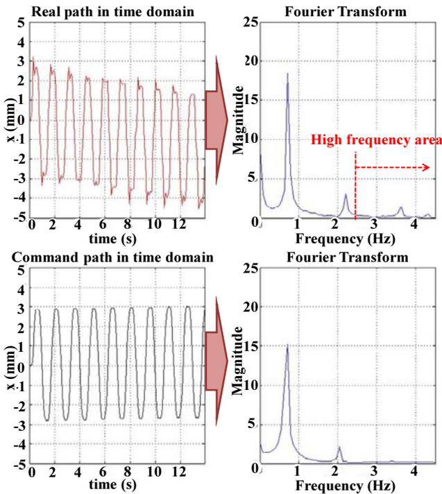
Fig. 10 Fast Fourier Transform of a trajectory at the end-effector
