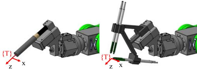
Fig. 1 Solid model of installation of measurement device instead of a welding torch at the end-effector of a welding robot
