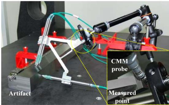
Fig. 4 Measurement set up of the measurement system with CMM
