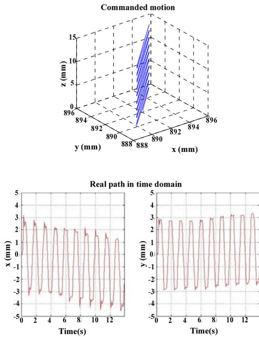
Fig. 9 The commanded motion and the measured trajectory in the x and y directions
