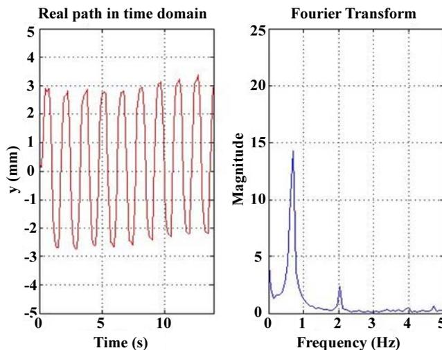
Fig. 12 Trajectory and FFT in the y-axis after gain tuning using the Taguchi method
