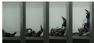
a) Photos of internal transitioning of Combot
