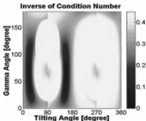
Fig. 11. Condition number plot of the actuator singularity configuration in the redundant case.
