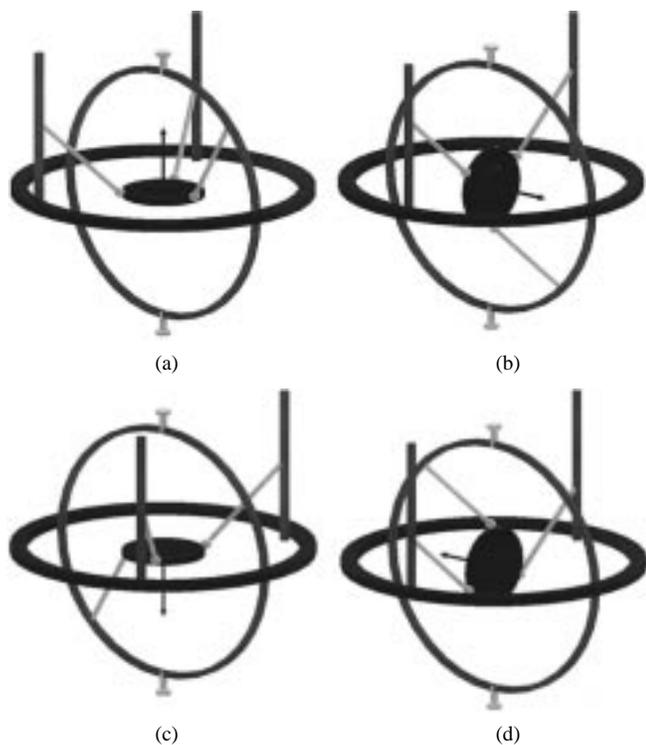
Fig. 2. Eclipse II mechanism and its 360° continuous rotational motions. (a) Rotation angle 0°. (b) Rotation angle 90°. (c) Rotation angle 180°. (d) Rotation angle 270°.
