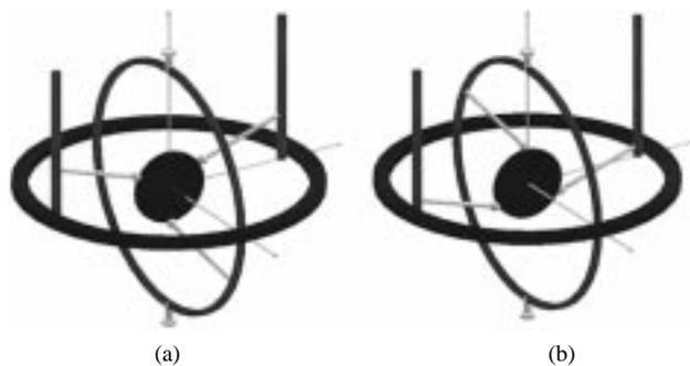
Fig. 6. Examples of the end-effector singular configuration. (a) Point A in Fig. 5. (b) Point B in Fig. 5.
