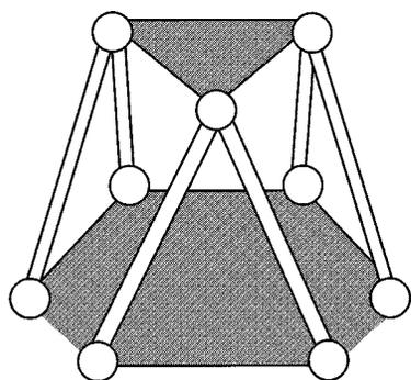
Fig. 1. Structure of Stewart–Gough platform.
