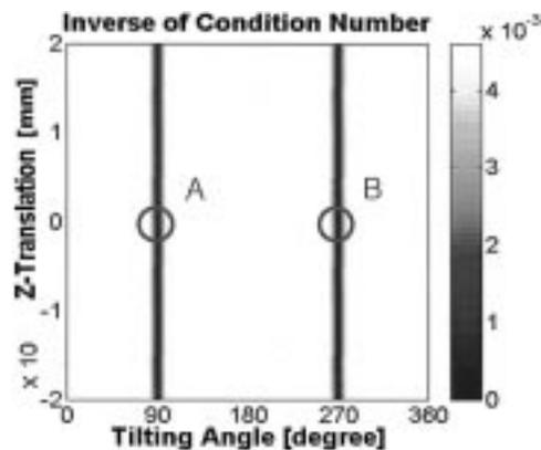
Fig. 5. Condition number plot of the end-effector singularity configuration.
