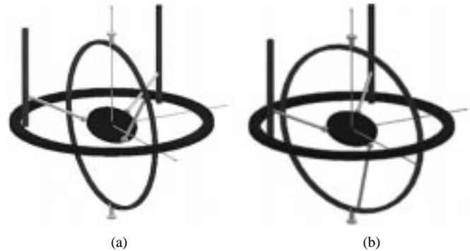
Fig. 10. Examples of the actuator singular configurations. (a) Point C in Fig. 9. (b) Point D in Fig. 9.
