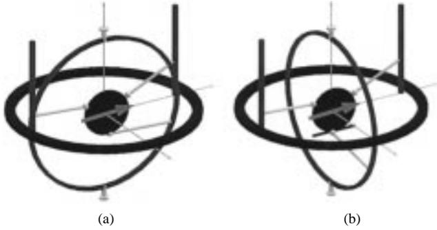
Fig. 7.  $y$ -direction motion of the Eclipse II. (a) 6 degrees of freedom Eclipse II. (b) 6+1 degrees of freedom Eclipse II.
