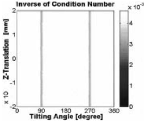
Fig. 8. Condition number plot of the end-effector singularity configuration of the 6+1 degrees of freedom Eclipse II.
