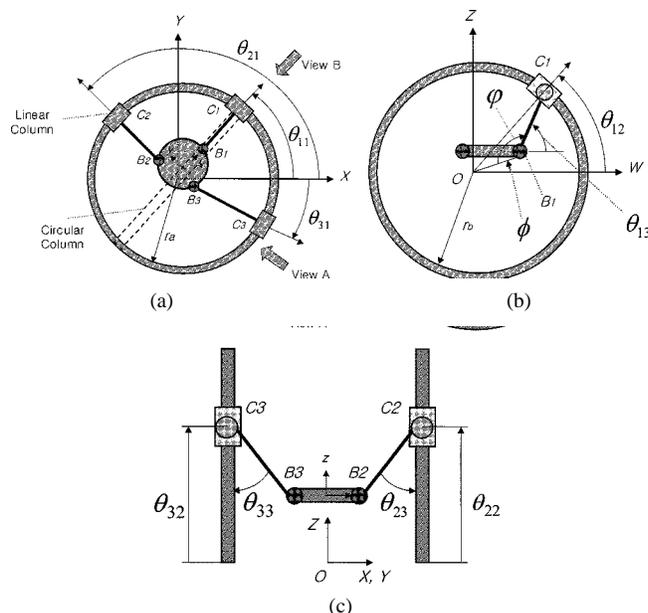
Fig. 4. Coordinate and joint convention. (a) Top view. (b) Side view A. (c) Side view B.
