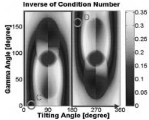
Fig. 9. Condition number plot of the actuator singularity configuration.
