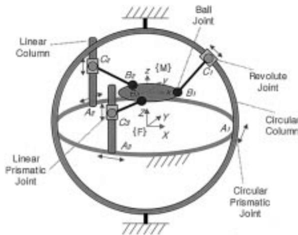
Fig. 3. Architecture of the Eclipse II mechanism.
