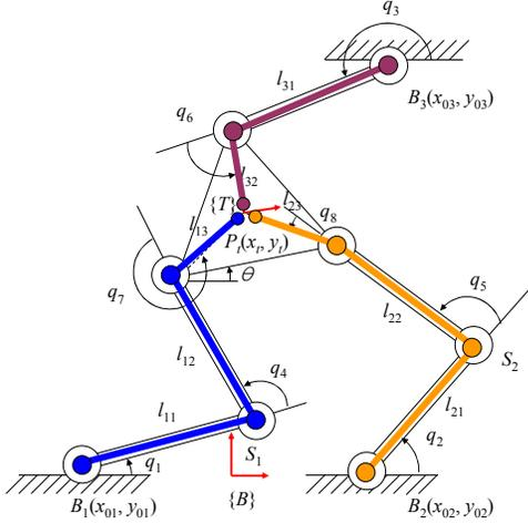
Fig. 1. Schematic of a 2-DOF parallel mechanism
