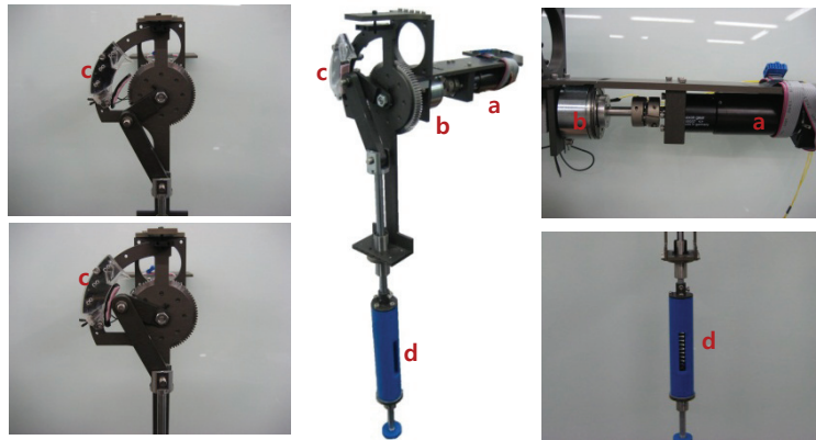
Fig. 3 Prototype: a) motor, b) clutch, c) holding equipment with switch, and d) spring linear guide.
