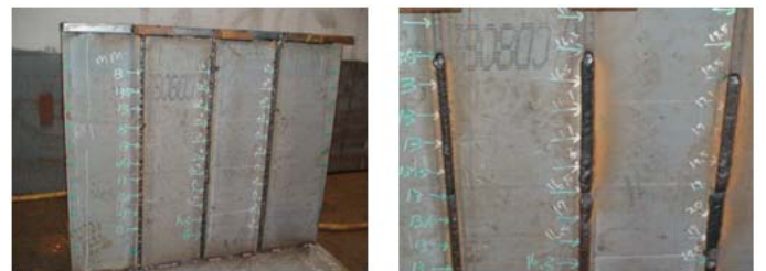
Fig. 7 Welding result using automatic welding robot
