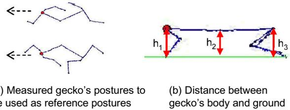
Fig. 4. Object function reference terms. Left upper: 1/4 cycle step posture of real gecko (used as 2/4 cycle pose for gecko model). Left bottom: 3/4 cycle step posture of real gecko (used as 4/4 cycle pose for gecko model). Right:  $h_1, h_2, h_3$  are heights from ground to neck, waist, bottom, respectively.
