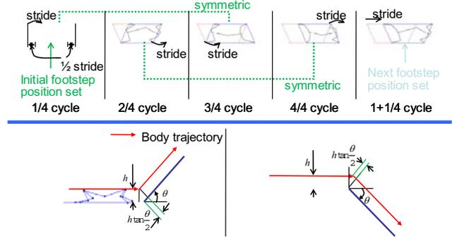
Fig. 6. Footstep rule. (Top: straight path footstep rule.) (Bottom: inclined/declined path footstep rule.)
