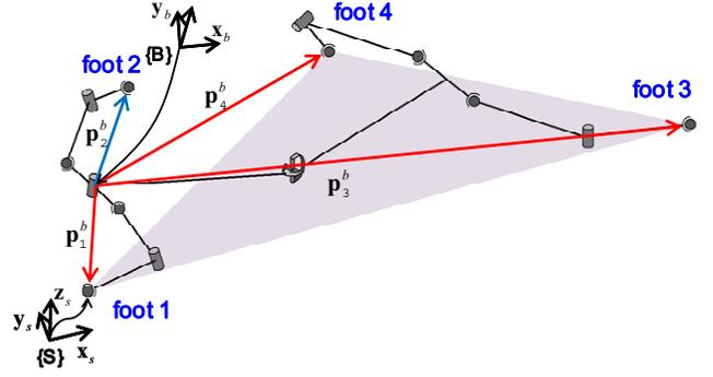
Fig. 3. Spatial frame and body frame on Gecko model.
