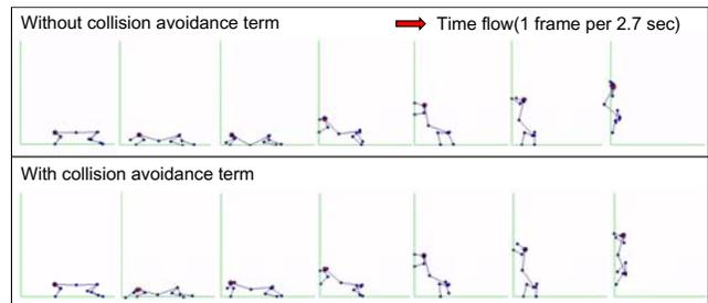
Fig. 9. Locomotion from horizontal to vertical plane of gecko model with and without collision avoidance term in object function.
