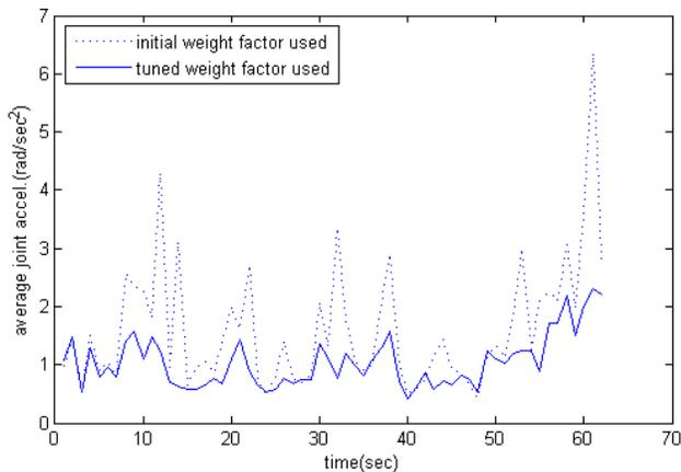
Fig. 10. Joint angular acceleration results with initial and optimal scalar factor.
