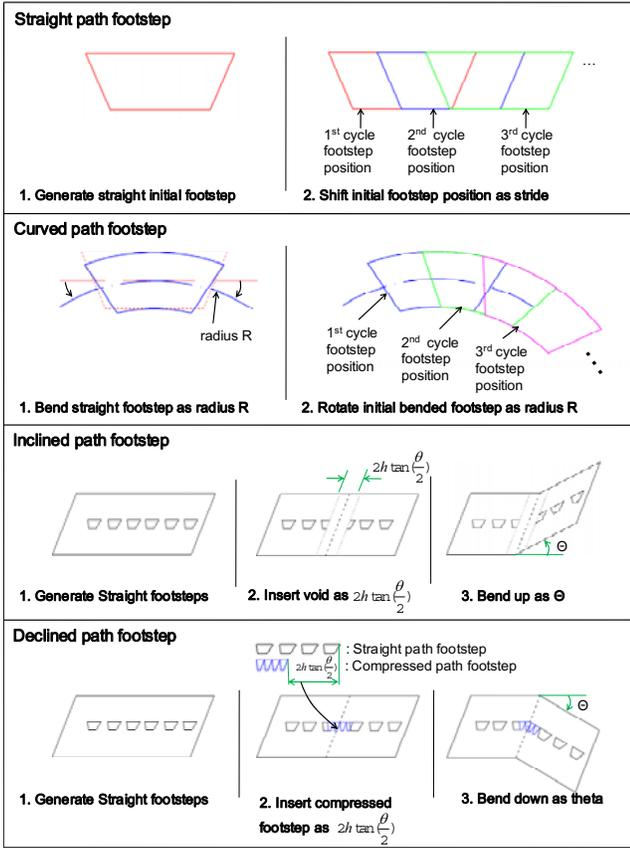
Fig. 7. Generation of straight, curved, inclined, declined path footsteps.
