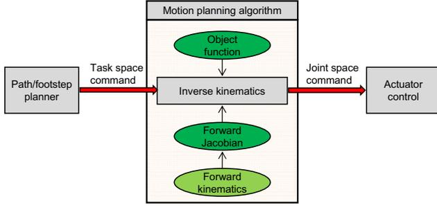
Fig. 2. Overview of motion planning algorithm.
