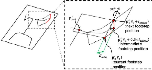
Fig. 5. Generation of swing foot trajectory.
