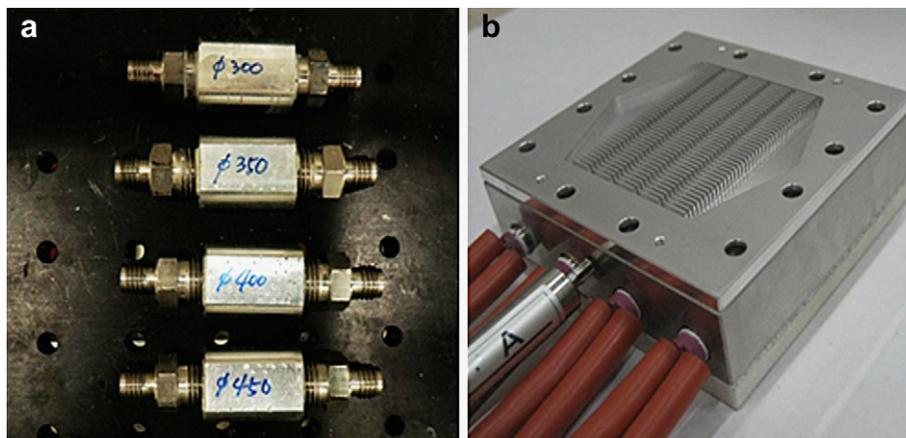
Fig. 6. Photo of (a) orifice samples, and (b) micro-evaporator with cartridge heaters.
