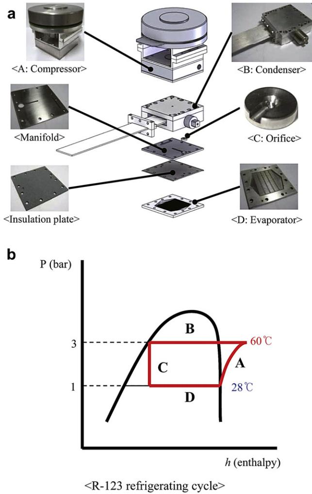
Fig. 1. (a) Concept of stack-type micro-cooler. (b) Refrigerating cycle of the cooler.
