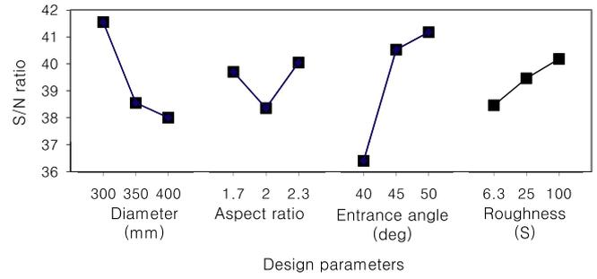
**Fig. 4.** Sensitivity analyses for each design parameter.
