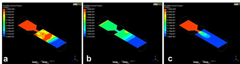
**Fig. 3.** Result of ANSYS simulation: simulation number 5 (the diameter = 350 μm, the aspect ratio = 2, the entrance angle = 50°, and the surface roughness = 6.3 S. a) NF1 (60 W, 30 mL/min), b) NF2 (80 W, 40 mL/min), c) NF3 (100 W, 50 mL/min).
