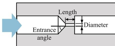
Fig. 2. Cross-section view of the orifice design.
