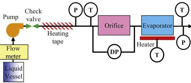
Fig. 5. Schematic diagram of experimental apparatus.
