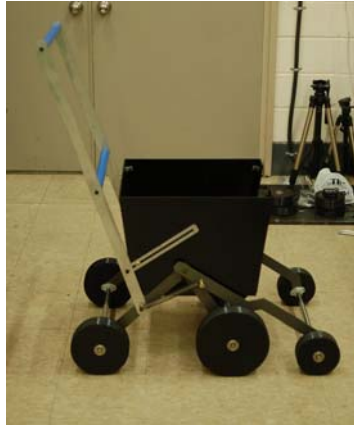
Figure 8. The photo of manufactured rocker-bogie cart (case 2)
