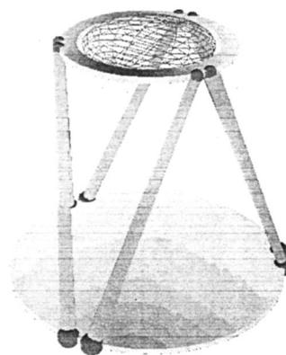
Fig. 2 Position manipulability ellipsoid of Stewart-Gough Platform in the home posture
