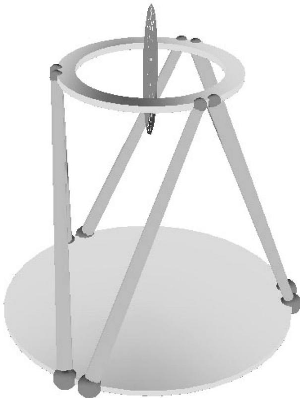
Fig. 4 Position stiffness ellipsoid of Stewart-Gough Platform in the home posture
