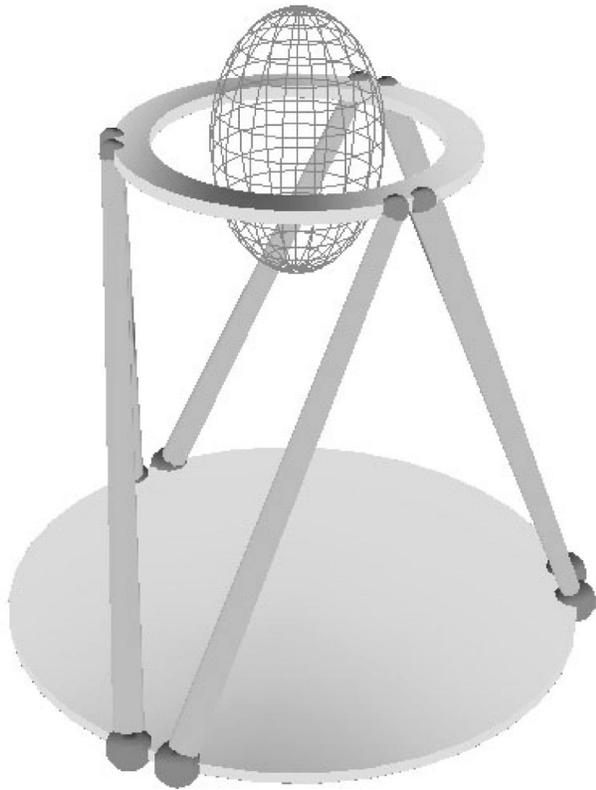
Fig. 3 Orientation manipulability ellipsoid of Stewart-Gough Platform in the home posture
