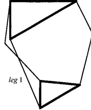
Fig.3 One singular configuration of the first kind of singularity: leg 1 is completely extended
