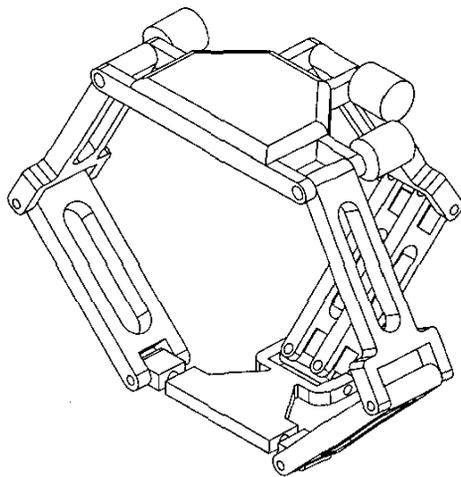
Fig.1 A *HALF* parallel manipulator with revolute actuators
