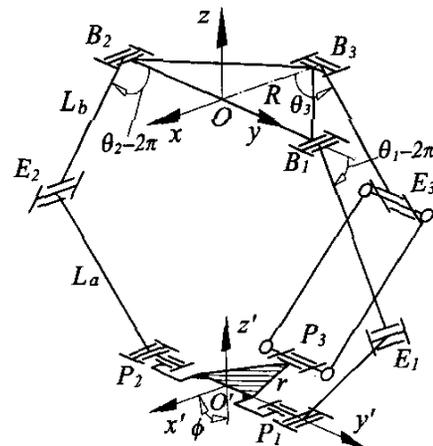
Fig.2 Geometric parameters of the manipulator
