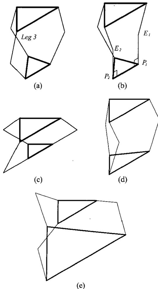
Fig.4 Some singular configurations of the second kind of singularity: (a) the lower link of the leg 3 is in the moving platform plane; (b)  $E_1P_1 \perp P_1P_2$  and  $E_2P_2 \perp P_1P_2$ ; (c) lower links of the first and second legs are collinear; (d)  $R = r$  and  $\theta_2 = \theta_1$ ; (e)  $R + L_b \cos \theta_1 = r$  and  $\theta_2 = \pi - \theta_1$ .
