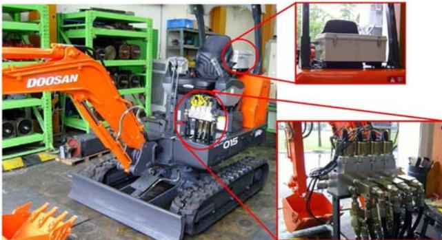
Fig. 4 The modified excavator with additional valves and a control box
