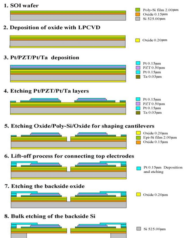
Fig. 10. Fabrication process of the microvalve.
