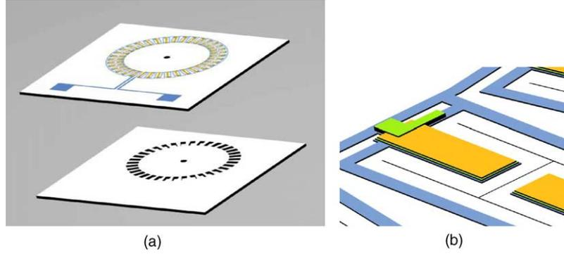
Fig. 1. (a) Schematics of the microvalve and (b) magnified view of a sub-unit.
