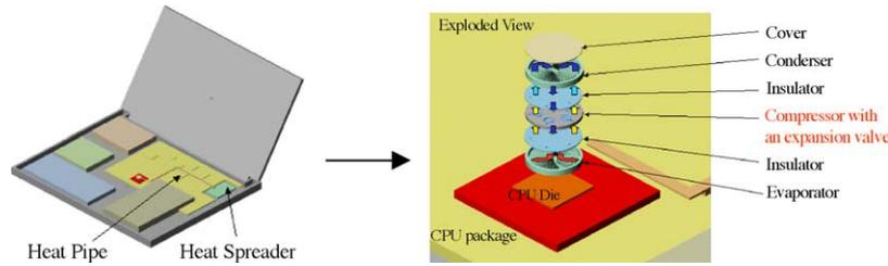
Fig. 8. Conceptual design of a micro cooler.
