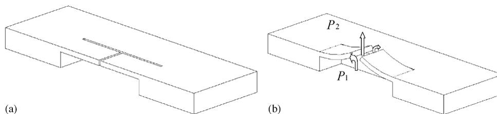
Fig. 3. Schematics of a working microvalve when (a) it is closed and (b) opened.
