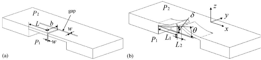
Fig. 6. Parameters of the microvalve model when (a) it is closed and (b) opened.
