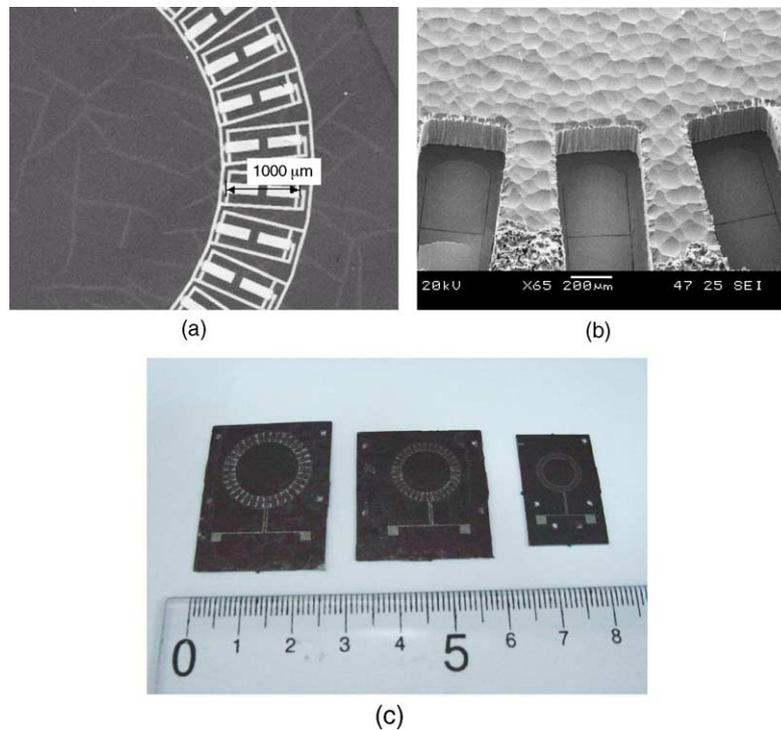
Fig. 2. The fabricated microvalves are shown by:(a) a front view SEM picture; (b) a backside view SEM picture; and (c) an overall picture of  $\Phi = 20, 15,$  and  $10$  mm-types from the left.
