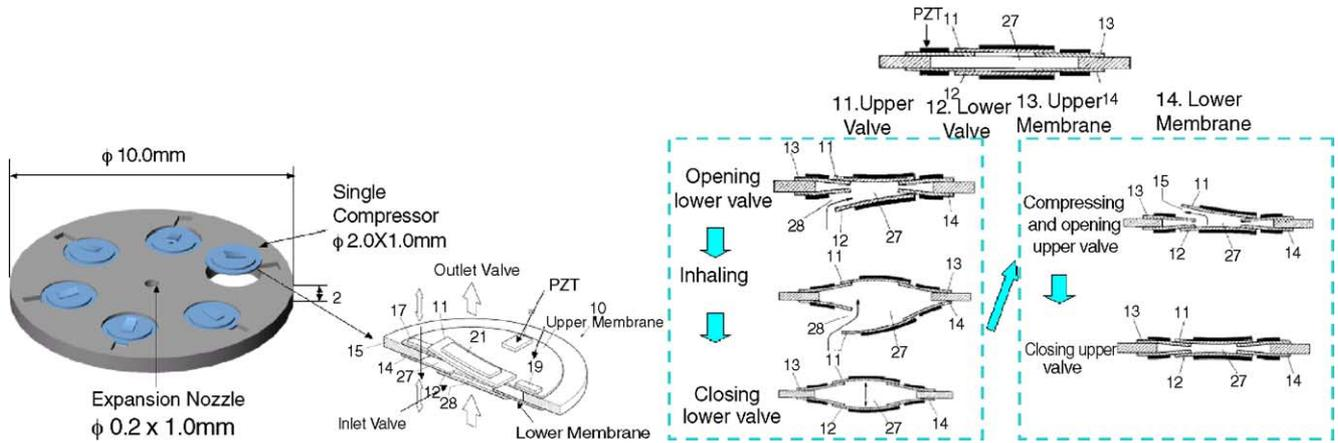
Fig. 9. (a) The conceptual design of the micro compressor and (b) working principle.
