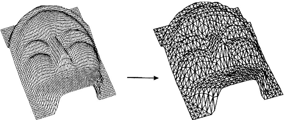
Figure 1. Comparison between surfaces generated by NURBS and polyhedron.
