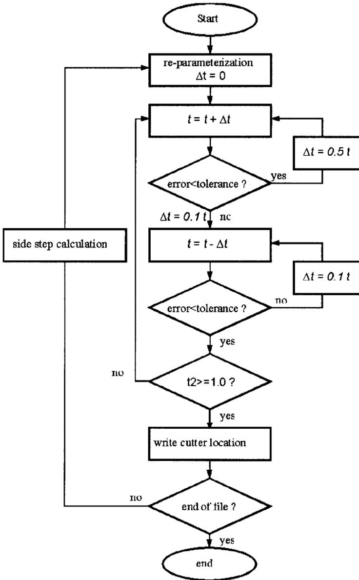
Figure 7. A simplified flow chart of the new variable step algorithm.
