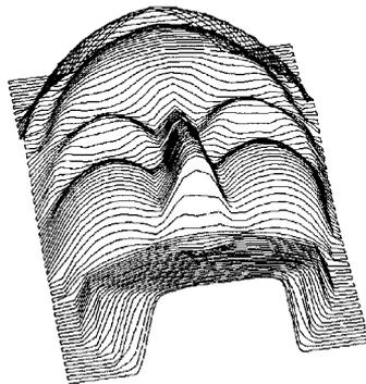
Figure 9. Generated tool path.
