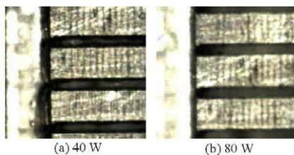
Fig. 10. Flow patterns of the 4th evaporator at 40 W and 80 W.
