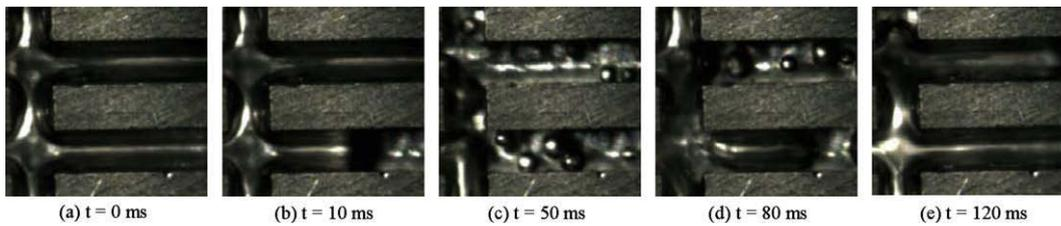
Fig. 8. Periodic change of flow pattern in the 6th evaporator at 40 W.
