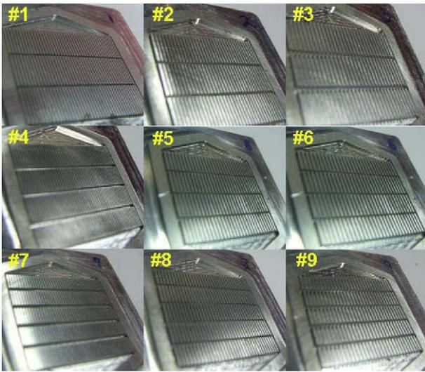
Fig. 5. Pictures of the micro evaporators constructed for the experimental studies.
