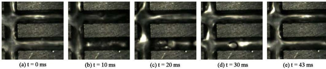
Fig. 9. Flow pattern of the 6th evaporator at 80 W.
