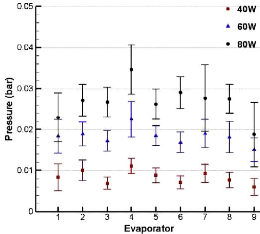
Fig. 3. Pressure drop in the micro evaporators.
