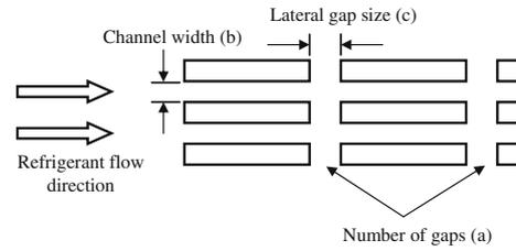
Fig. 4. Definition of the design parameters.
