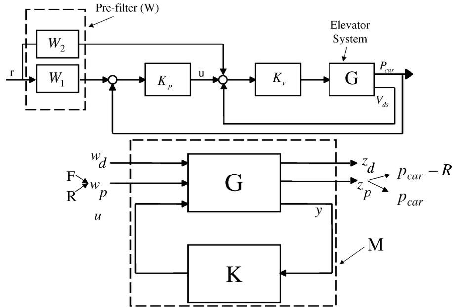
Fig. 4. Top: block diagram a sequential control setup; bottom: schematic diagram of the framework for  $\mu$  robustness analysis.
