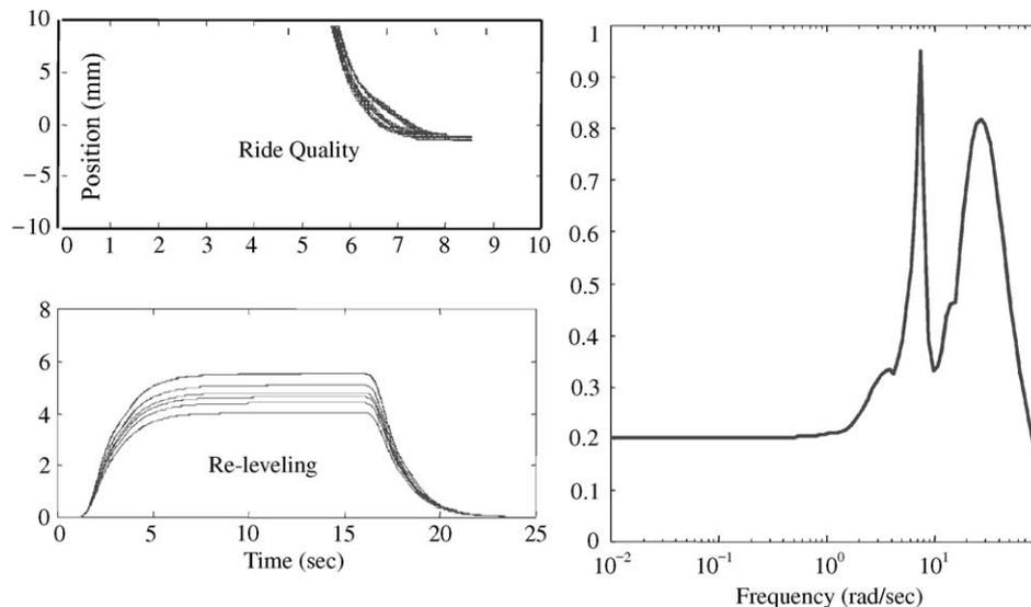
Fig. 6. Top-left: simulation of vertical ride of the elevator system as a function of time and with parametric variation; bottom-left: simulation of re-leveling response of the elevator system as a function of time and with parametric variation; right:  $\mu$  robustness analysis plot.
