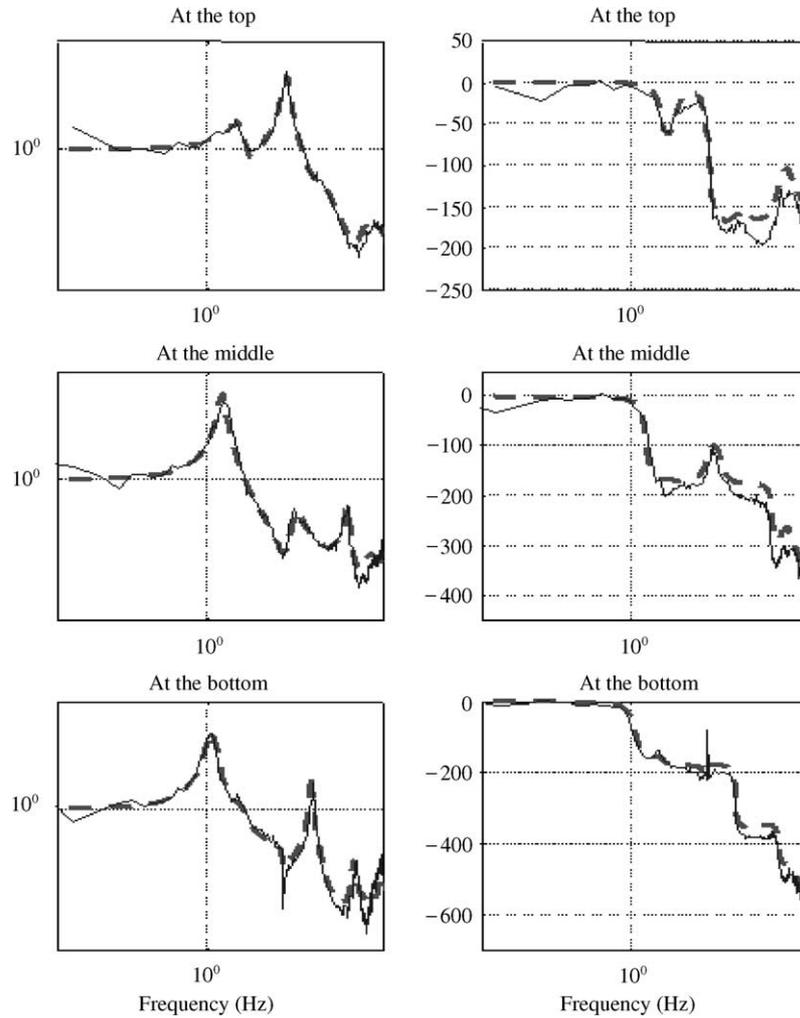
Fig. 1. Model-validation results with sinusoidal (dots) and random inputs (dashed) for the elevator system; comparison of physics-based model (solid) with experimental data; illustration of movement of modes with elevator position.
