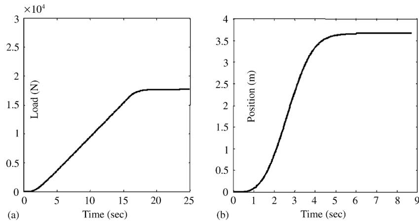
Fig. 3. (a) Typical load profile for simulating re-leveling performance; (b) a one-shuttle run profile used as a reference trajectory dictation for evaluating vertical ride quality.
