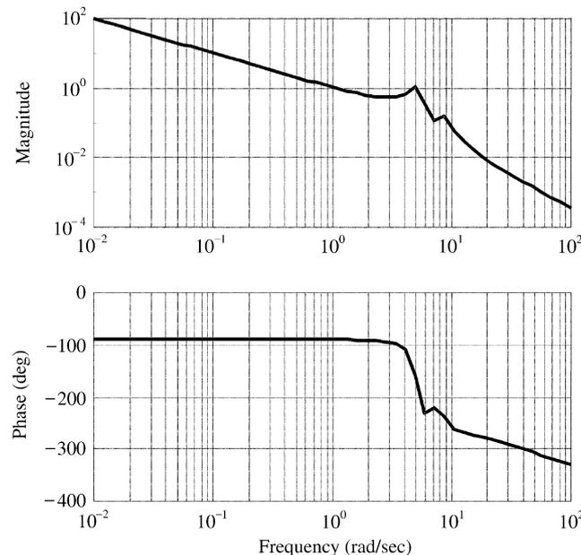
Fig. 5. Frequency domain magnitude and phase plots for the transfer function between the torque actuation and car position when the drive sheave loop is closed.
