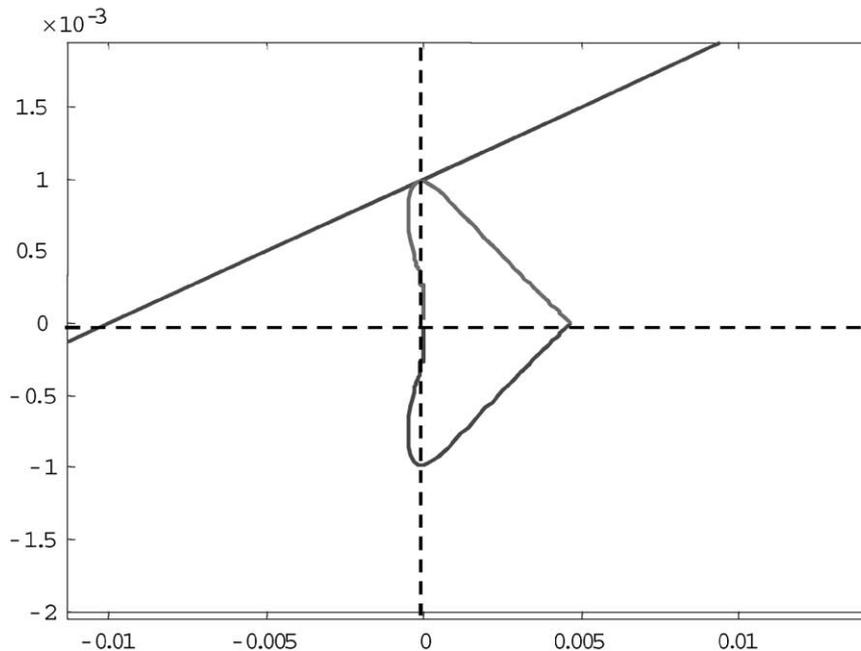
Fig. 7. Popov plot for the case where only the state equation for the car changes with position.
